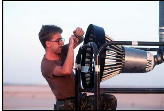
Preparing a KC-135 for refueling a probe equipped receiver
