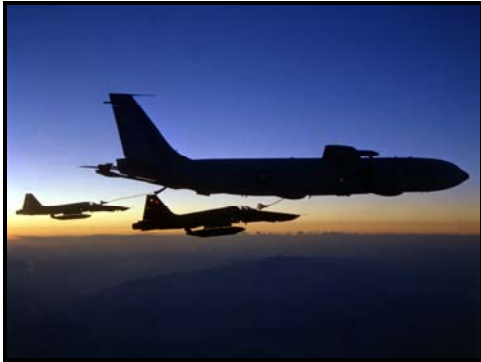
Multinational refueling with tanker capable of both boom and drogue refueling
